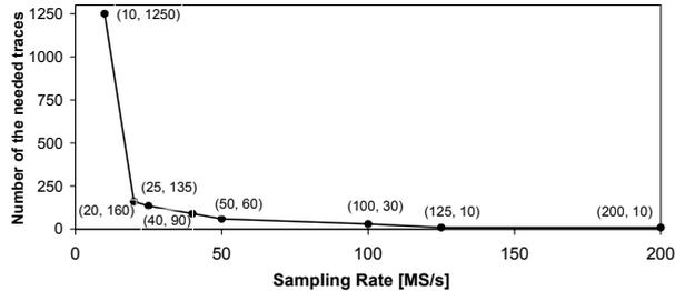
**Fig. 7.** Number of measurements required for revealing the secret key of a HCS201 IC in a DIP package as a function of the sampling rate. The numbers in parentheses give the exact coordinates of the points.
