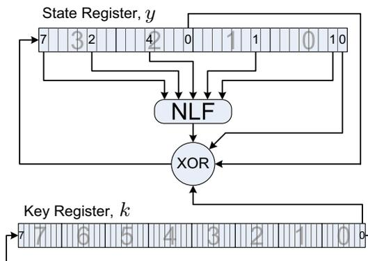
**Fig. 1.** Block diagram of the KEELOQ encryption
