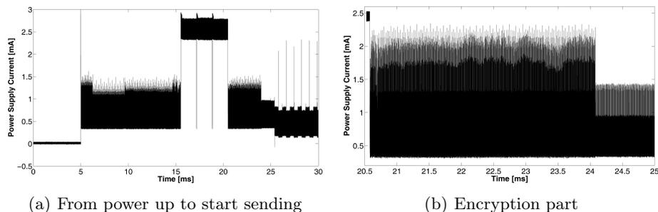
**Fig. 5.** Power consumption traces of a HCS module
