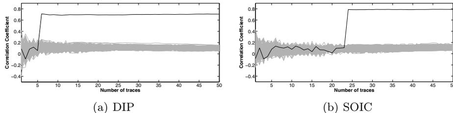
**Fig. 6.** Correlation coefficients of key hypotheses of HCS201 ICs as a function of the number of measured traces.
